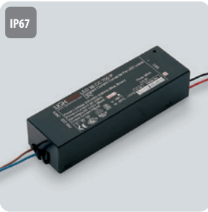
L18350C IP67 18W/350mA constant current driver PSU for use with KKDC eSEN Constant Current LED driver, 350mA Black metal casing L133mm W40mm H31mm
