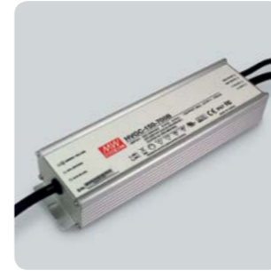
KKM150350110-CC 350mA KKM150700110-CC 700mA 1 channel 1-10V Dimmable constant current PSU Standards: cRUus/CE/CB/FCC
