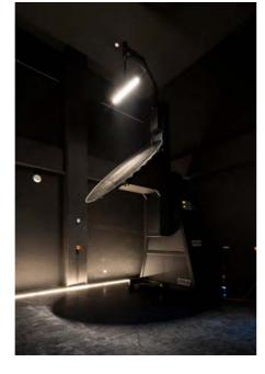
Unlike the more common Type A/B goniometers, Type C is the requirement for UL Certified testing facilities.
