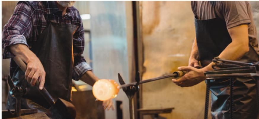
*The last step is the refinement: to create the wanted shape and texture, the almost finished product is cut, pulled and striped with special tools. Any excess is also taken out.*
