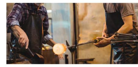
The last step is the refinement: to create the wanted shape and texture, the almost finished product is cut, pulled and striped with special tools. Any excess is also taken out.
