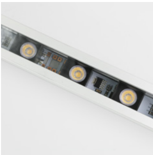
BL 12 Clear cover 12° lens + Louvre (UGR 4H 8H <10.0/<10.0) W25.0/H26.5mm (W0.98/H1.04")
