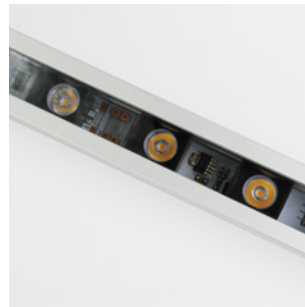
BL 25 Clear cover 25° lens + Louvre (UGR 4H 8H <10.0/<10.0) W25.0/H26.5mm (W0.98/H1.04")
