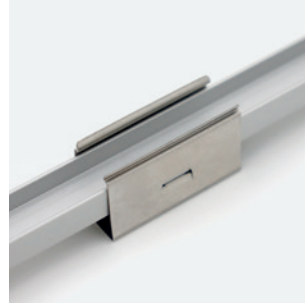
KKCP-13 Lock clip (allow 2 per metre/40in) S/Steel finish L25/W10.8/H14.5mm (L0.98/W0.43/H0.57")
